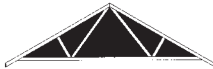
Trusses are prefabricated with metal plates at the joints
